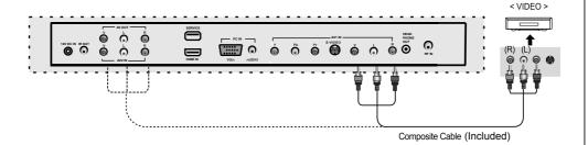
Connect the LCD TV'S Composite In terminal to VCR's Composite OUT terminal using the included Composite cable. (Make sure the color of the terminals and the color of the cable are the same)
